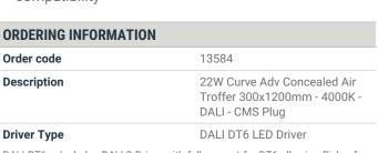
DALI DT6  $\sim$  Includes DALI-2 Driver with full support for DT6 allowing flicker free dimming with compliant DALI-2 Application controllers.
